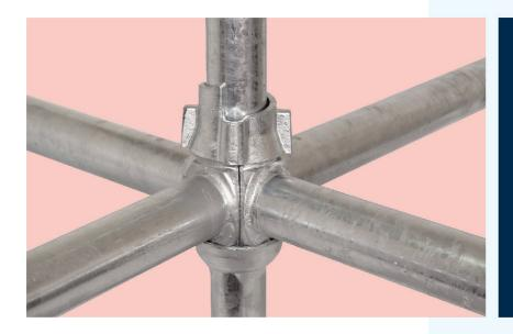
The locking device is formed by two cups at 500mm c/c, bottom cup welded to vertical tube and a movable upper cup. The forged blade ends of horizontal are located into the bottom cup, the upper cup is moved down and rotated to secure the horizontal in place and tightened by a hammer blow to give rigid connection.
